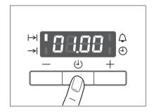
2. Using the End time → function, set the time at which the dish should be ready. In this case 14:05:00.
